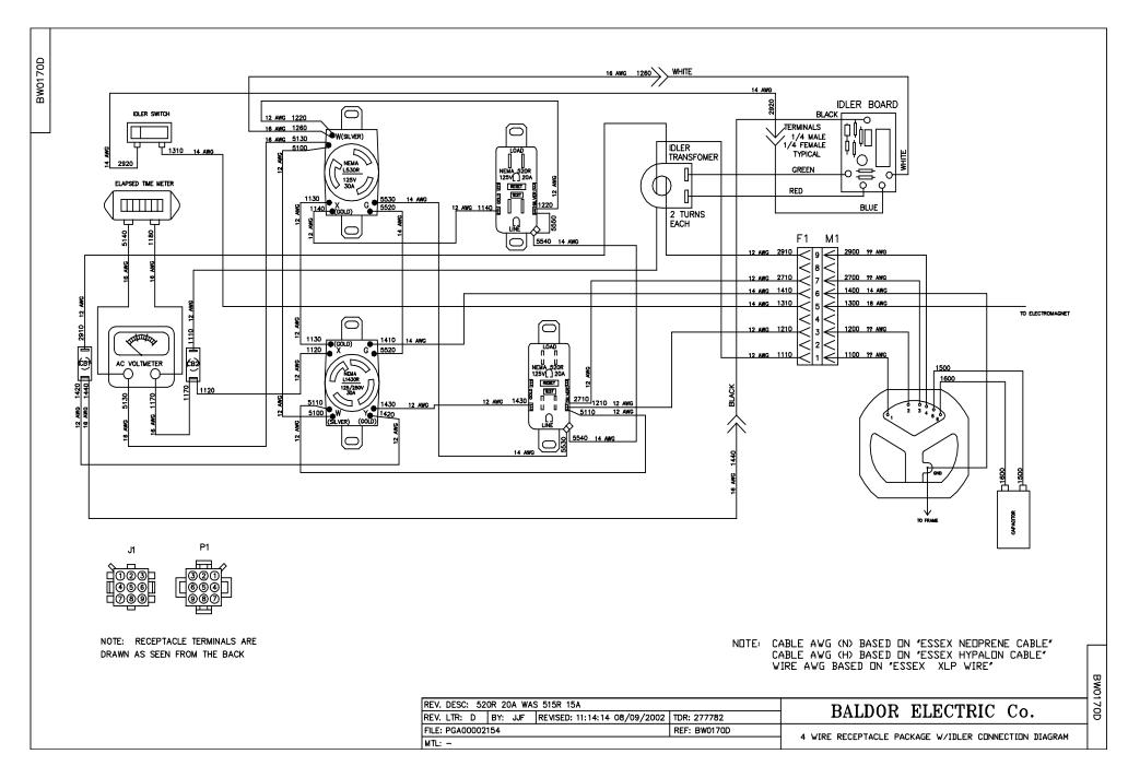
Wiring Diagram OHV85E
